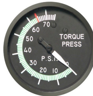
27-3007-4 0 to 75 PSI Green Arc From 0 to 64.4 Red Line at 64.4
